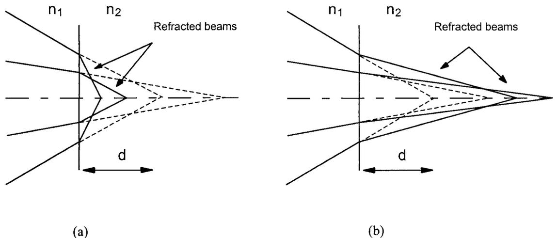
Fig. 1. Schematic diagram of beams being refracted on an interface between two media: (a)  $n_1 > n_2$  and (b)  $n_1 < n_2$ .
